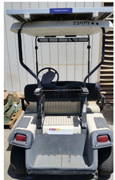
Figure 2- One of the first fully “solarized” golf carts in CSUDH’s campus fleet
